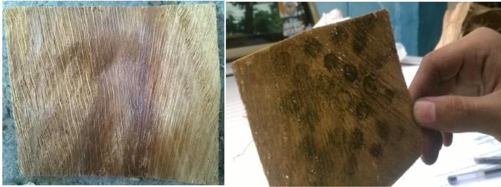
Figure 6: Physical appearance of coconut spathe fibers. before air filtration, (b) after air filtration
