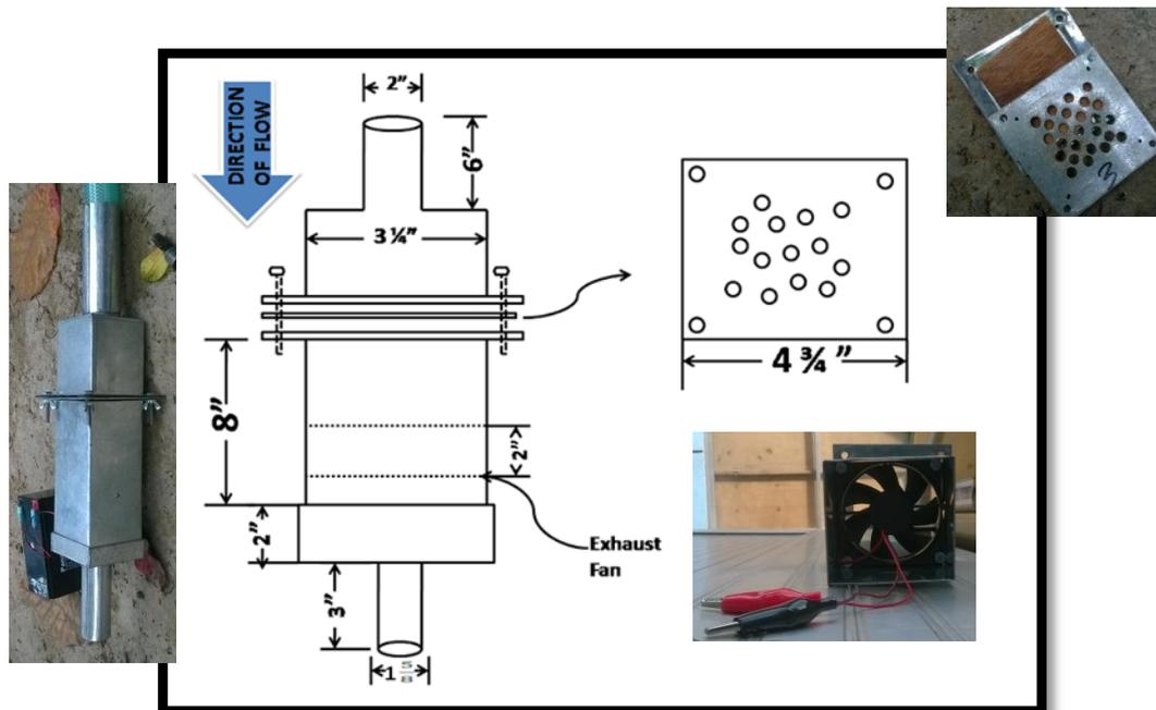
Figure 3: Air filter case prototype
