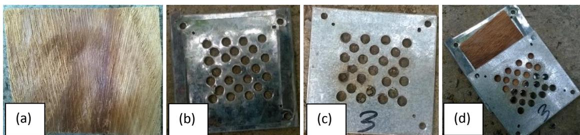
Figure 2: Improved Filter Media. (a) spathe fibers, (b) metal plate-front view, (c) metal plate- back view, (d) filter media
