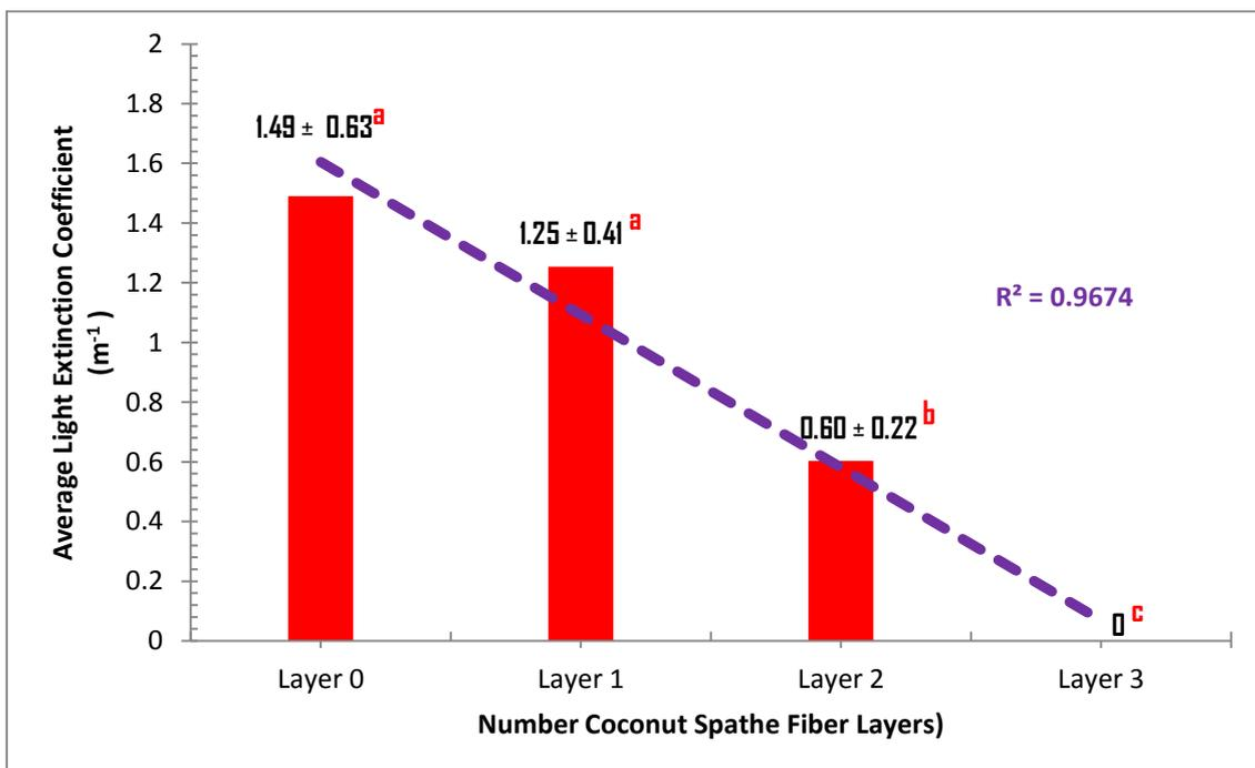
Figure 5: Light Absorption Coefficient as a function of Coconut Spathe Fibers
