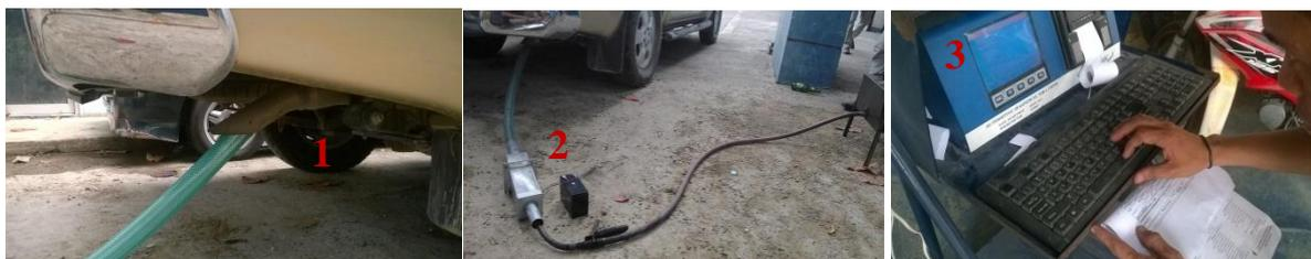
Figure 4: Standard Opacity Test using a Digital Opacimeter at Land Transportation Office- Region VII
