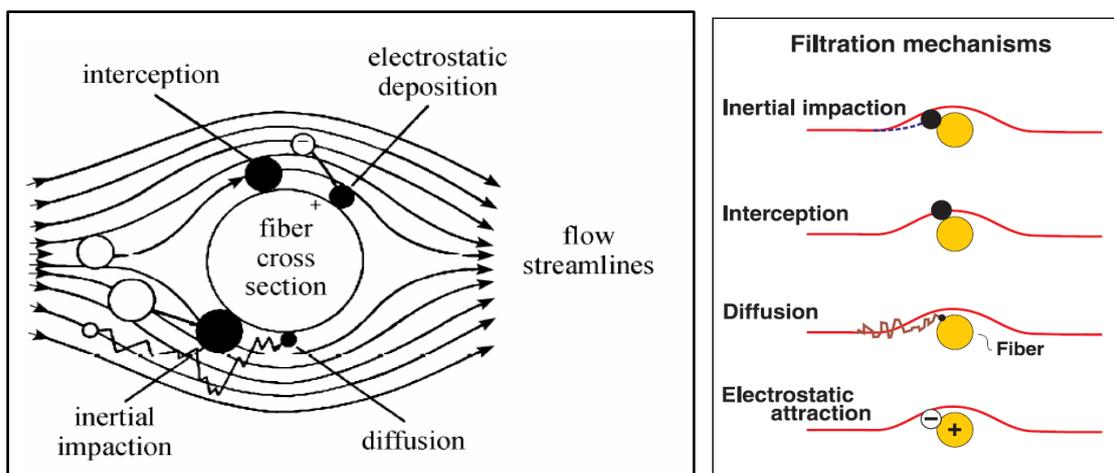
Figure 7: Four primary filter collection mechanisms using fibrous substances (Chuanfang, 2012)
